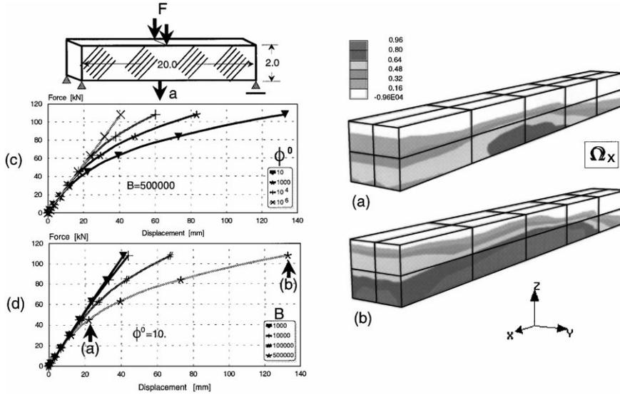
Fig. 4. Simply supported beam model: damage evolution.
