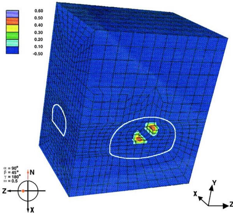
Fig. 6. Distribution of maximum principal active damage: loading 1.
