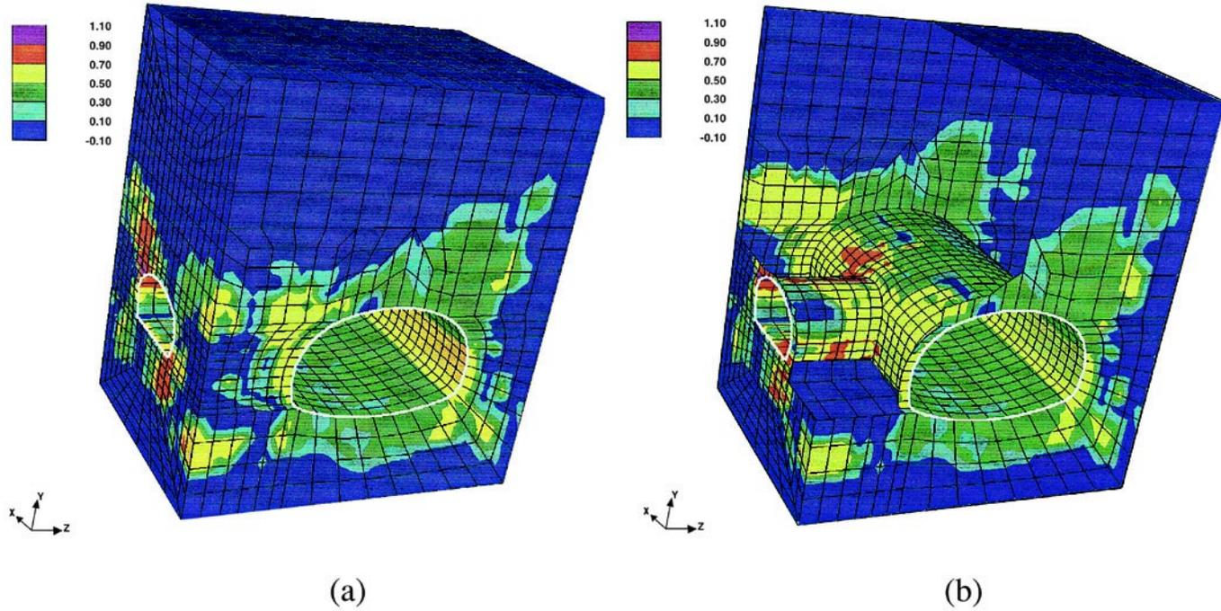
**Fig. 9.** Damage for 3 joint sets (a) before and (b) after damage: propagation: loading 10.
