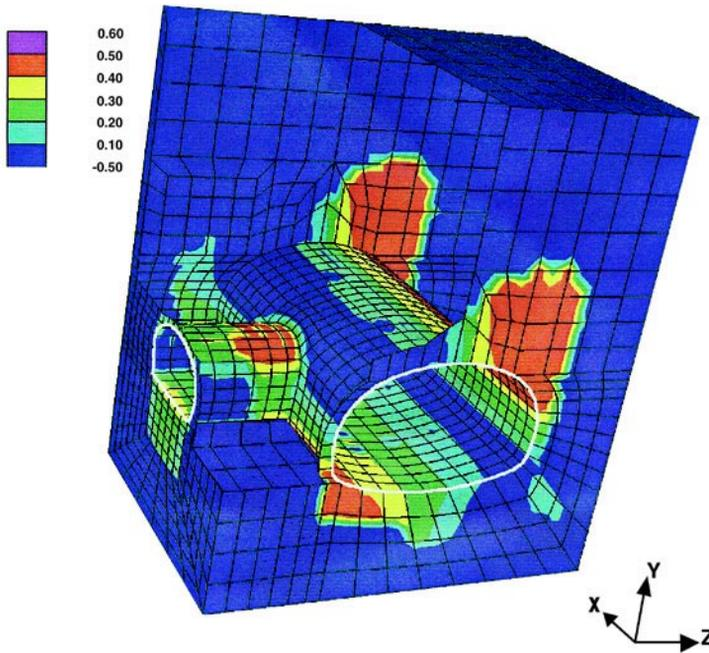
Fig. 8. Distribution of maximum principal active damage: loading 10.
