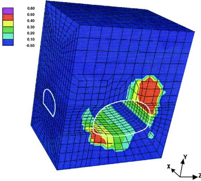
Fig. 7. Distribution of maximum principal active damage: loading 7.
