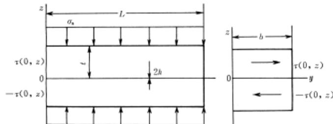
Figure 1 Double-shear-plates bonded by cohesive layer
