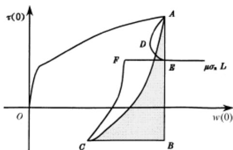
Figure 3 Schematic diagrams for snap-back behavior
