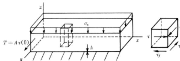
Figure 2 Shear beam model
