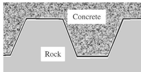
**Figure 1.** Illustration of artificial joints between concrete dam and rock foundation
