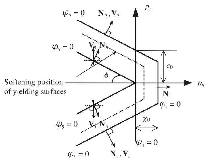
Figure 3. Illustration of piece-wise linear plastic yielding surfaces
