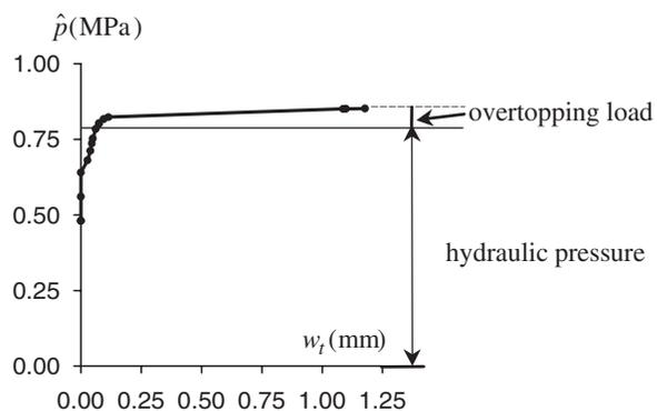
(a) Response of load vs crack mouth opening in tangential direction
