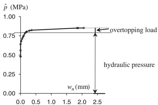
(b) Response of load vs crack mouth opening in normal direction
