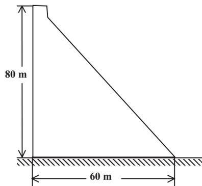
Figure 5. The geometry of the benchmark gravity dam
