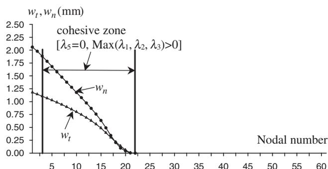
Figure 7. Distribution of crack opening displacements along the length of the interface
