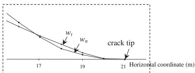
Figure 8. Distribution of displacements in the cohesive zone (enlarged local view)
